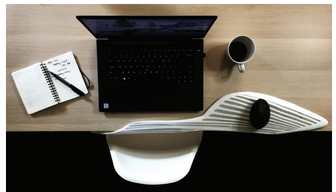
9 The piece's primary structure consists of a rigid 3D printed wing-like form that wraps around the desk to maintain its stability and positioning. An ultra-thin layer of nylon encloses the top of the piece, serving both as a smooth continuous surface to serve as a functional mouse pad and as a permeable seal that stops the scent infused hydrogel beads from falling out.
